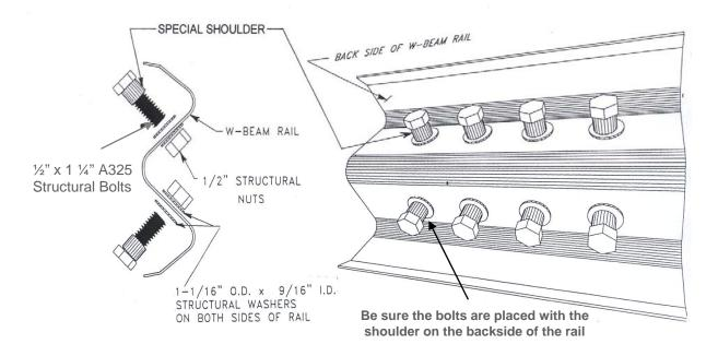
Figure 8. Installation of Cable Anchor Bracket Shoulder Bolts
