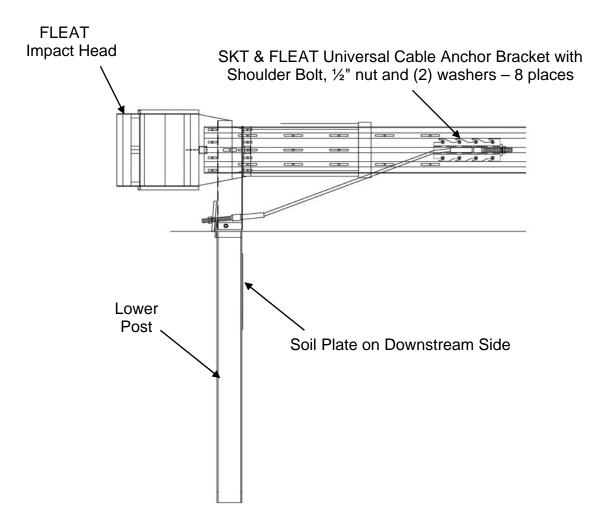
**NOTE**: Be sure the 5/8" x 9" hex bolt at Hinged Post #1 is on the upstream side of the post.
