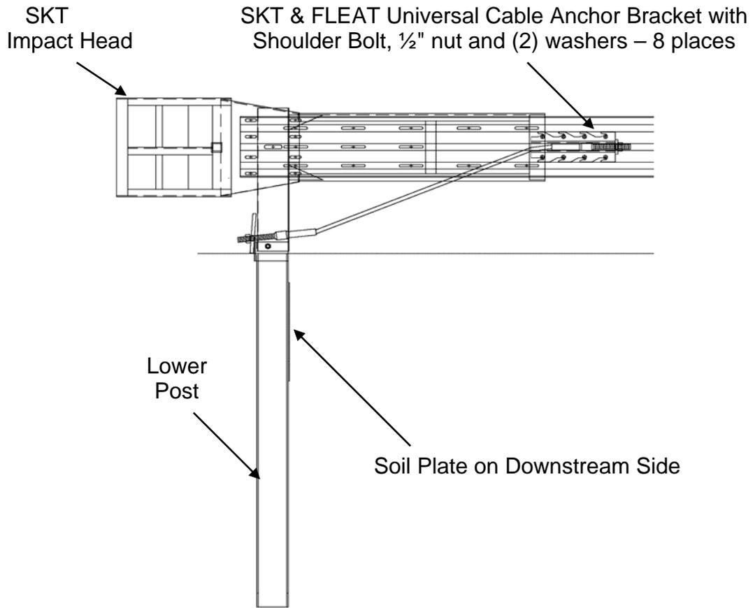
**NOTE:** Be sure the 5/8" x 9" hex bolt at Hinged Post #1 is on the upstream side of the post.
