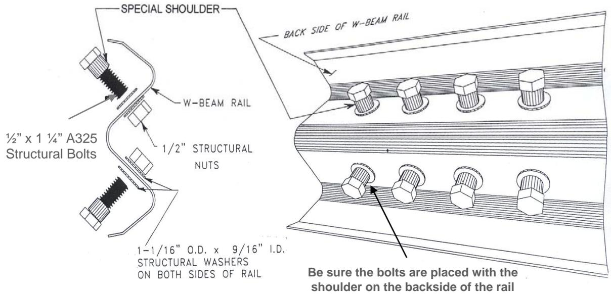
**Figure 8. Installation of Cable Anchor Bracket Shoulder Bolts**
